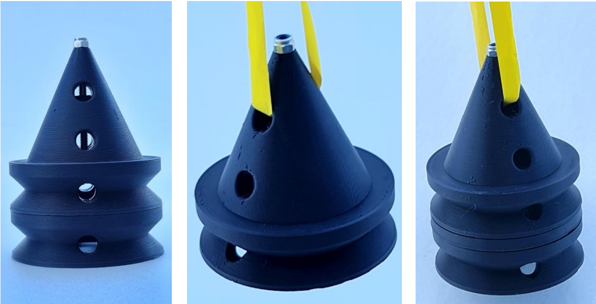
Figure 4: Pictures of the stacked cones 100 g (left), unstacked 50 gr (middle) and stacked cones with dummy weight between (200 g).
